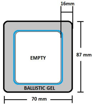
Fig. 3. Side View of Mold Schematic
