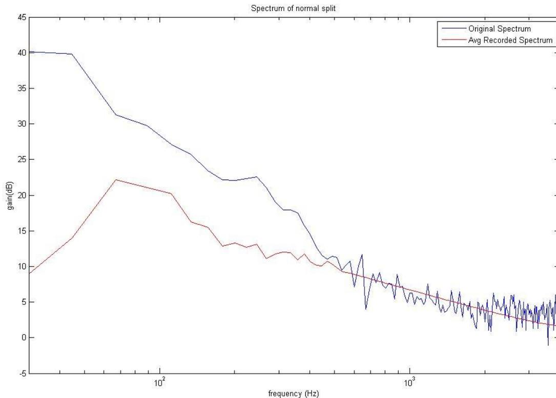
Fig. 12. Spectrum of Normal Split, Original vs. Average Recorded
