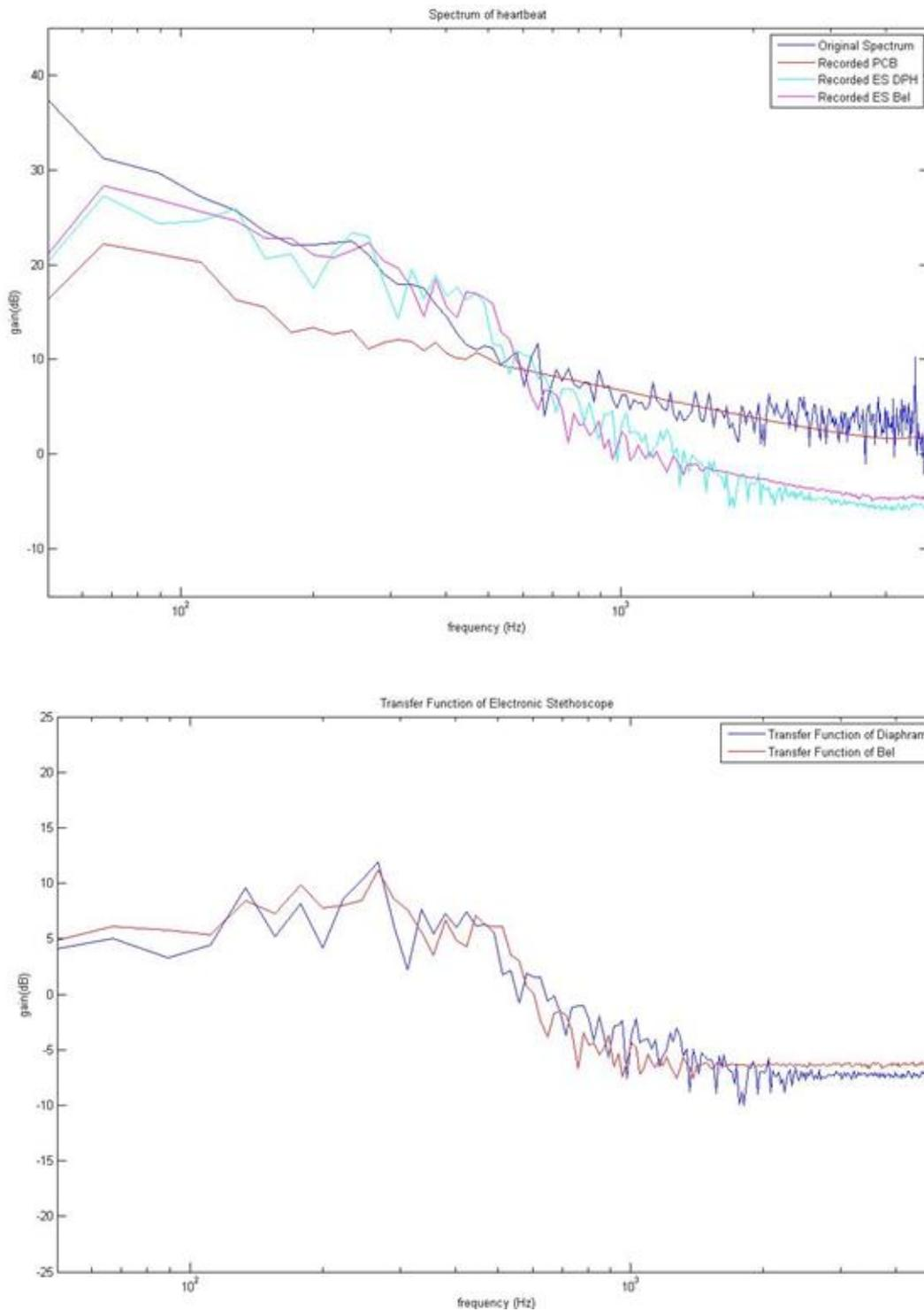
Fig. 16. Spectra and Transfer Functions of Heartbeat Sound
