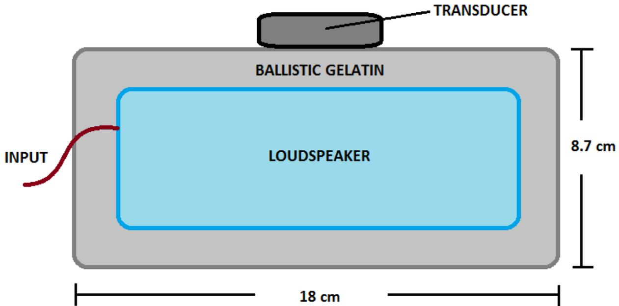
Fig. 1. Front View Schematic of Respiratory Sounds Simulator
